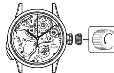
4. Push the crown back in to the normal position simultaneously with a time signal.
