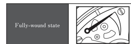
※The crown cannot be turned further when the mainspring is fully wound to prevent overwinding of the mainspring. Do not try to forcefully turn the crown as this may damage the watch.
