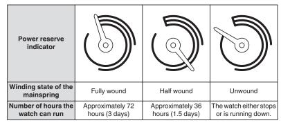
\* The crown cannot be turned further when the mainspring is fully wound to prevent overwinding of the mainspring. Do not try to forcefully turn the crown as this may damage the watch.
