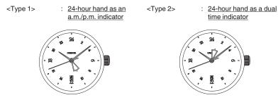
Simply using the 24-hour hand to show the 24-hour time as an a.m./p.m. indicator. (This is the standard usage type for the 24-hour hand.)
